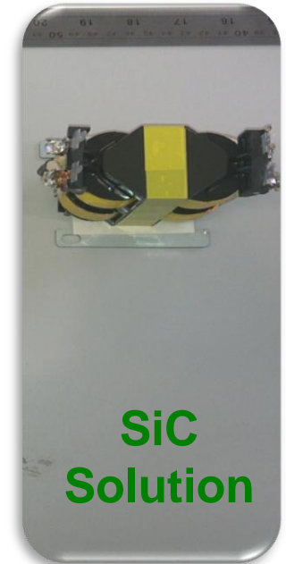
Transformer at 100 kHz
